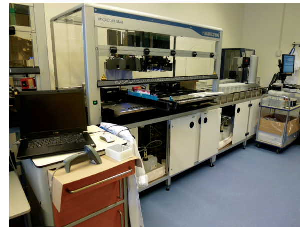
The large robot in the DNA lab that isolates DNA from blood
